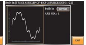
Fourier Series Synthesized Waveform
