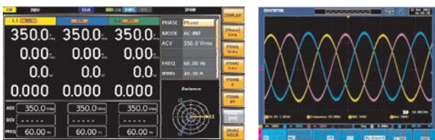
AC Balanced Three-phase
