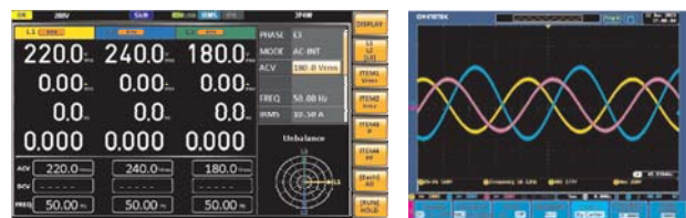
AC Unbalanced Three-phase
