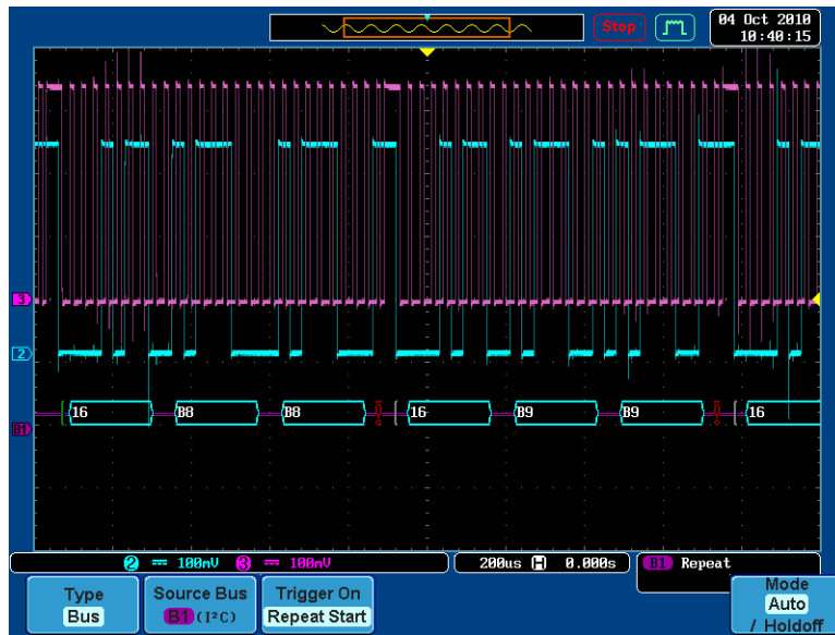
Fig. 7 Illustration of the GDS-3000 I 2 C decoding
