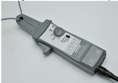
Figure 2: Connecting the GCP-300 current probe.
