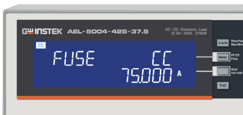
Turbo : OFF, Fuse mode Test result screen
