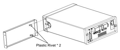
Step 3 - forPlace the unit along with front plate combined into thesingle unitbottom cover of rack mount followed by tightening the M4\*12screws in the front end as the following figure shown.
