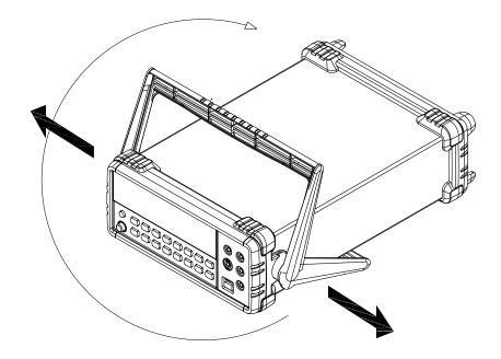
2. Further remove both the front and rear protective rubber casings away from unit as the figure below shown.
