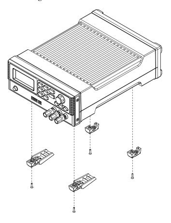
Step 2 - forConnect the front plate with unit in parallel with fastening the<br/>plastic rivets firmly.
