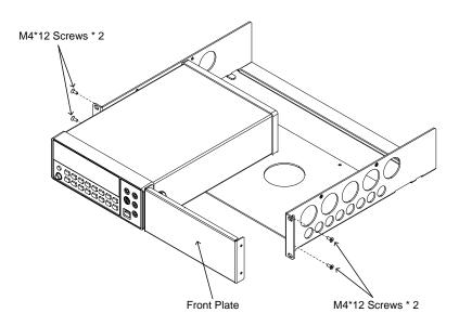
Step 4 - forPut the top cover onto the rack mount followed by fasteningsingle unitthe M3\*4 screws in the 2 sides as the following figure shown.The rack mount is completely assembled with unit.
