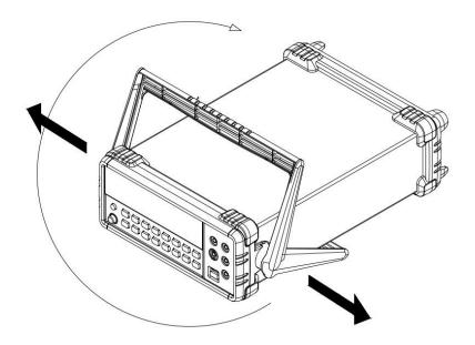
2. Further remove both the front and rear protective rubber casings away from unit as the figure below shown.
