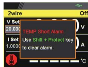
Red: The Alarm of Short Circuit Occurs From Temperature Measurement
