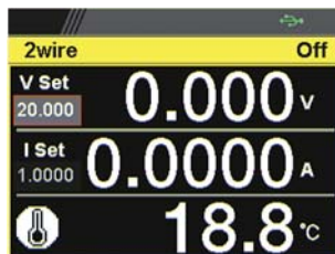
White: Temperature Control on with GTL-205A Connected
