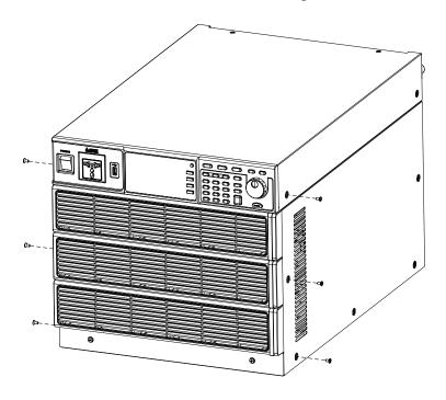
3. Screw the left bracket (62RA-430HP101) to the left side panels of the APS-7300 and right bracket (62RA-430HP201) to the right side panel of the APS-7300 using the six (594B-W4012NS1) screws as shown in the below diagram.
