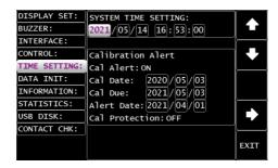
Year setting  $2000 \sim 2099$ Month setting  $01 \sim 12$ Date setting  $01 \sim 31$ Hours setting  $00 \sim 23$ Minutes setting  $00 \sim 59$ Seconds setting  $00 \sim 59$
