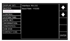
Press the ENTER soft-key to enter the Interface setting followed by using the scroll wheel to select the Interface options.
