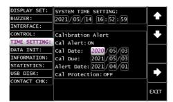
Cal Date  $2000 \sim 2099$   $01 \sim 12$  $01 \sim 31$   Press the UP/DOWN arrow softkeys to move the cursor to the Cal Due setting followed by using the scroll wheel to set the Cal Due setting, which indicates next due date for calibration.
