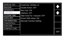
3. Press the ENTER soft-key to enter the Control By setting followed by using the scroll wheel to select the following options.
