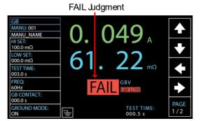
2. The FAIL judgment will be held on the display until the STOP button is pressed. Pressing the STOP button will return the tester back to the READY status.
