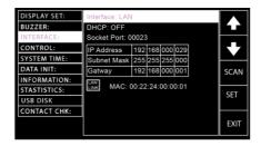
When pressing the SACN soft-key, the unit will scan the LAN card setting thoroughly. In fact, the unit automatically scans at once every time when Interface is changed to LAN setting.
