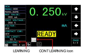
5. After pressing the START button, the GPT-15012 unit will perform the CONTACT CHK before running a MANU test. If the measured current is lower than the reference value by user-defined percentage, the "OPEN" status appears on the screen.
