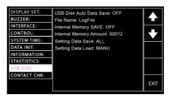
Press the ENTER soft-key to enter the USB Disk Auto Data Save setting followed by using the scroll wheel to turn on or off the setting, which automatically saves the test data into the inserted USB disk when enabled.
