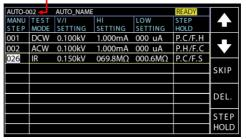
4. After the previous steps, return to the AUTO-001 test page followed by pressing START button for automatic test. The AUTO-002 test will ensue from the end of AUTO-001 test. The continuous AUTO tests are thus established perfectly.
