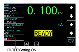
4. Press the START button to perform ACW/DCW mode test with the filter setting ON.
