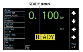
Press the START button when the tester is in the READY status. The manual test starts accordingly and the tester goes into the TEST status.
