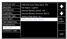
Press the USB LOAD soft-key to load the selected data from the USB disk.
