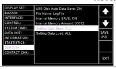
Press the SAVE USB soft-key to save selected data into USB disk. The saved data will be named AUTODATA.txt, MANUDATA.txt & SYSTDATA.txt respectively within the directory GPT1X000/SET\_DATA.
