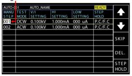
Press the STEP HOLD soft-key to bring the cursor to the STEP HOLD setting field.
