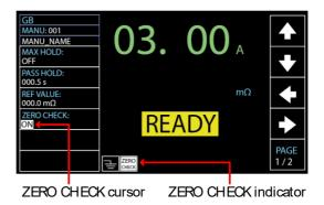
4. Press the START button to perform the zero check. The resistance of the test leads, after the ZERO CHECK has finished, will be added into the REF VALUE field as the display shown below.
