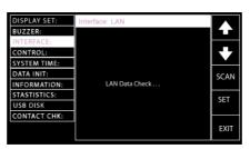
If LAN card with network setting is scanned properly, the "LAN LINK" icon appears. If not, however, the icon doesn't appear.
