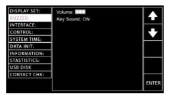
Press the ENTER soft-key to enter the Volume setting followed by using the scroll wheel to set the Volume level.
