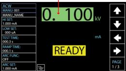
2. Use the scroll wheel to set the test voltage or ampere level.
