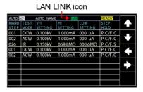
When LAN setting is Not scanned properly and Interface is set as LAN, the "LAN OPEN" icon shows as the following figures.
