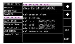
Press the ENTER soft-key to enter the Year setting followed by using the scroll wheel to select the Year setting for system. Also, repeat the actions for the rest month, date, hour, minute and second settings.
