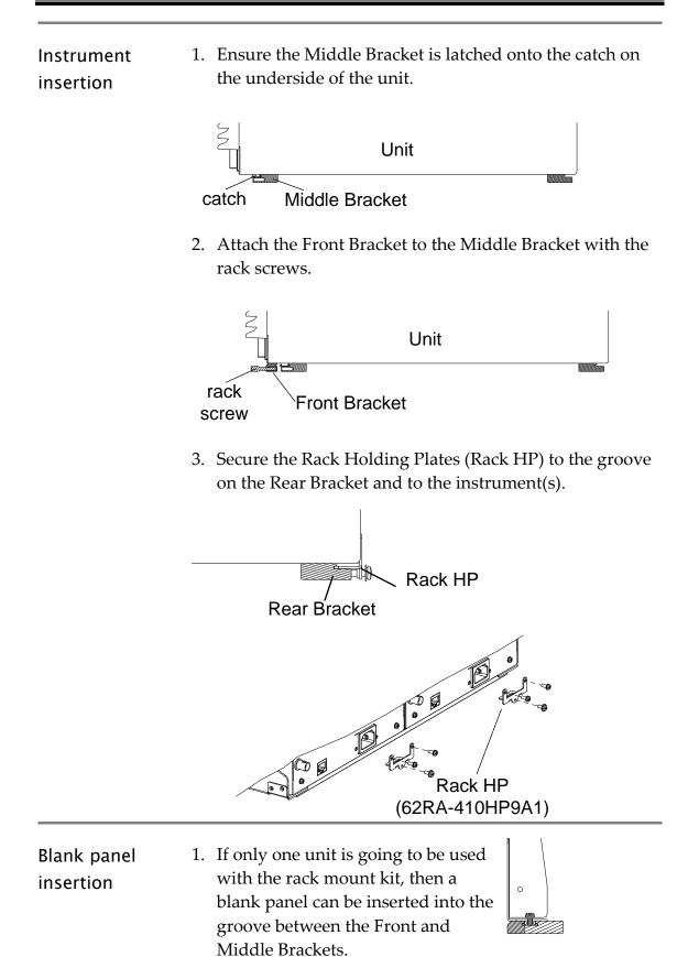
2. Secure the panels with the PMS-W-3\*8 screw.
