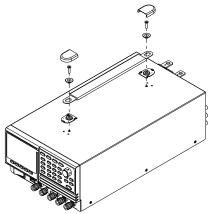
2. Remove the feet from the underside of the unit.
