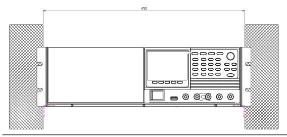
The angle brackets are used to support the bottom of the rack.
