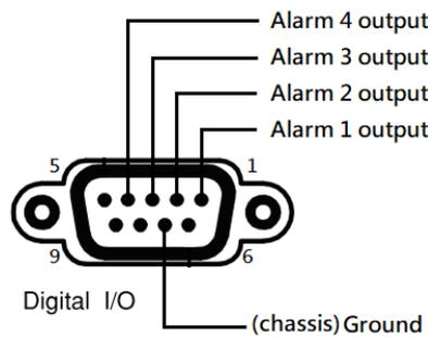
**Pin1-4** Alarm output pins
