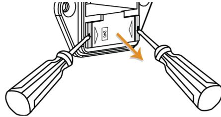
2. The fuse socket appears. The “240” symbol within the hole on fuse socket indicates the line voltage is positioned as 240V.
