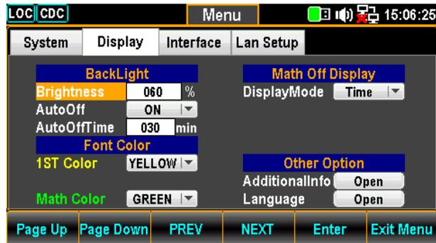
2. Press the NEXT key repeatedly or scroll the Knob key to move to the BackLight - AutoOff field.
