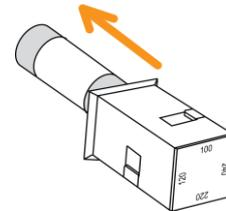
5. Restore the fuse holder with new fuse back to the fuse socket. Ensure that the correct line voltage shows within the hole of the fuse socket per requirement.
