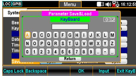
5. Use the Left/Right and +/- keys or scroll the Knob key to move the cursor to desired word followed by pressing the F5 (Input) key or Knob key to input the word.
