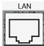
It accepts a LAN cable for remote control. For Ethernet remote control details, see page 190.
