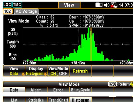
2. When the “CH” is selected for *ViewMode* (F3) key, scroll the *knob* key to navigate through channels.
