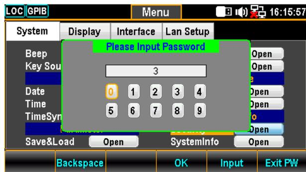
3. Use the Left/Right and +/- keys or scroll the Knob key to move the cursor followed by pressing the F5 (Input) key or the Knob key to input the password.
