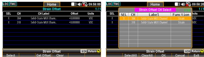
Get Offset Press to get offset value(s) for selected channel(s) immediately. The offset values are displayed for each selected channel accordingly.
