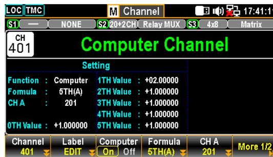
2. Press the *(x)TH* (F1) key to select a coefficient order (0TH, 1TH, 2TH, 3TH, 4TH, 5TH) followed by pressing the *TH Value* (F2) key to configure parameters for each coefficient order.
