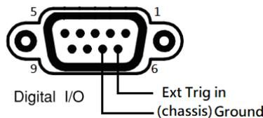
**Pin6** External Trigger Input pin
