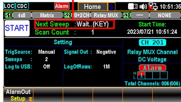
External It indicates a trigger signal received from the rear panel to start each sweep for a scan course. Press the *TrigSignal* (F2) key to configure the polarity of external signal in either Pos or Neg.
