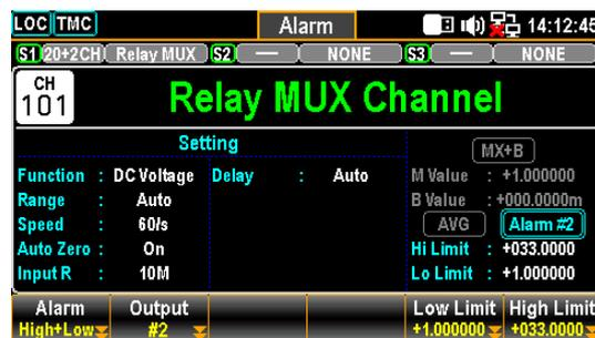
Press the *Alarm* (F1) key to select an alarm limit(s) mode for the select channel.
