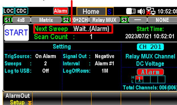
F2 (Time) key to set interval When Time of TrigSource is selected, press the key to specify a time interval.
