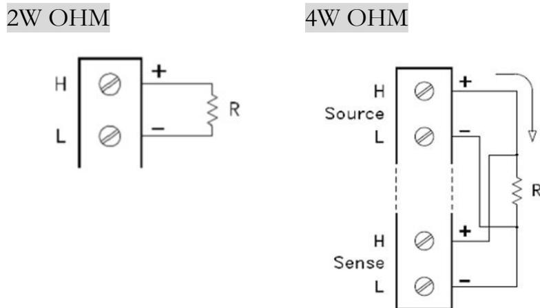
F4 (Range) key to specify range Press the key to enter Range menu and select a target range for 2W OHM and 4W OHM measurements individually. The Auto indicates a range, which is based on the source input, is selected automatically. It is sometimes results in, compared with manual select range, slower measurement. Also, using the *Range keys* can select range promptly.
