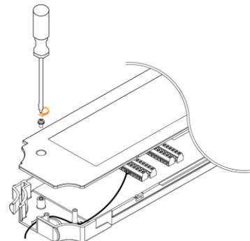
4. Insert the module into one of the module slots from the rear panel of DAQ-9600 unit.
