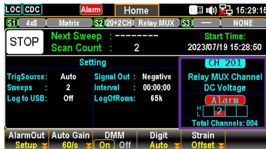
The set low limit of alarm #2 is triggered
