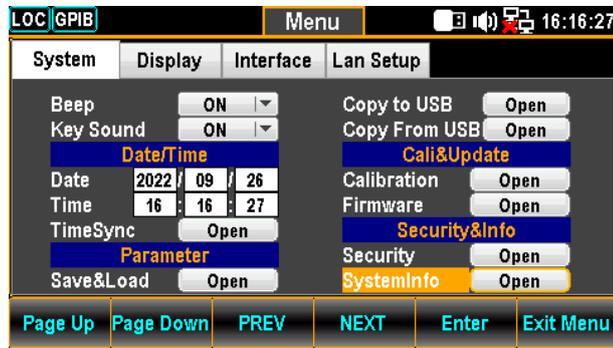
2. Press the F5 (Enter) key or Knob key to enter the System Information where all the critical contents are exposed for check.
