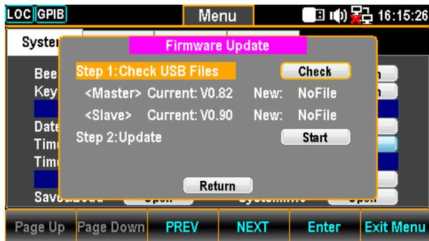
**Firmware Update** **Update Process** Prior to update, make sure if the required firmware file is stored within the flash drive plugged into the USB port on the front panel. Also, user can check the current Master and Slave firmware version respectively in this menu.
