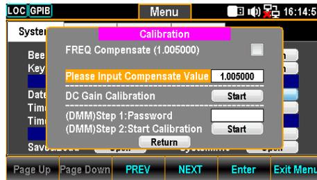
2. Use the Left/Right keys to move the cursor followed by pressing the F5 (Enter) key to save the frequency compensation coefficient. The value changes as the figure shown below.
