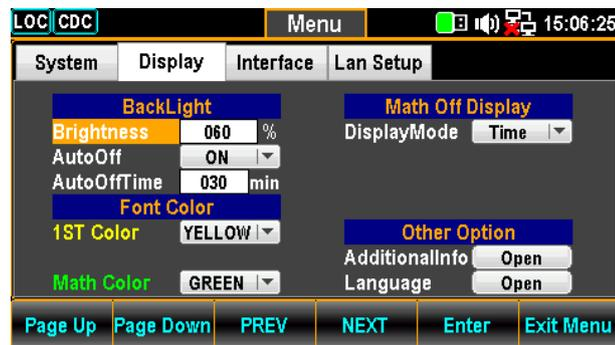
2. Press the NEXT key repeatedly or scroll the Knob key to move to the BackLight – AutoOffTime field.
