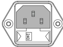
Accepts the power cord. AC 100/120/220/240V  $\pm 10\%$ , 50Hz / 60Hz  $\pm 10\%$ .
