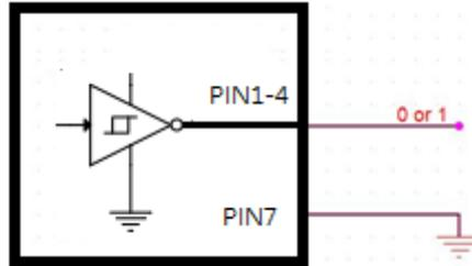
Pin5 EOM (End Of Measurement) signal Output. Activates when compare measurement is over. It is also available in other measurements.
