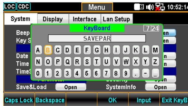
3. Use the Left/Right and +/- keys or scroll the Knob key to move the cursor followed by pressing the F5 (Input) key or the Knob key to specify a name for parameters.
