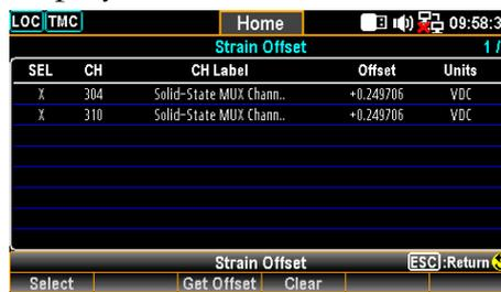
Clear Press to clear the offset value(s) of selected channel(s). The offset value(s) on the list are returned to 0 instantly after execution.
