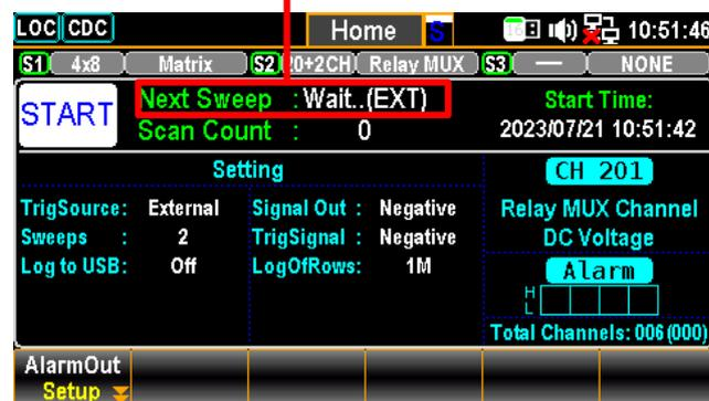
On Alarm It indicates a sweep starts when an alarm is detected from the set channel. Press the *On Alarm* (F2) key to specify which alarm (1-4) is used to report on the select channel.
