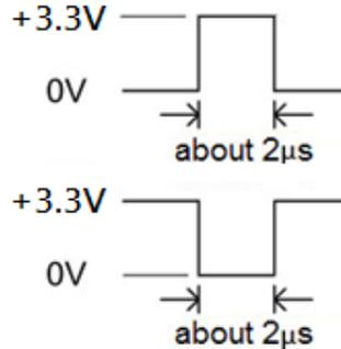
Pin6 External Trigger Input. Accepts external trigger signals. For using external signals.
