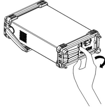
2. Use 2 fingers to grip curve areas of both right and left sides on slot cover and gently pull outward so as to remove slot cover from DAQ-9600 unit.
