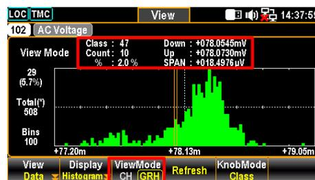
4. Due to readings are not updated with the live scan in histogram display, press the *Refresh* (F4) key to update live readings when a scan course is ongoing.
