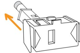
4. Further pull the fuse out of the fuse holder and replace it with a new fuse.
