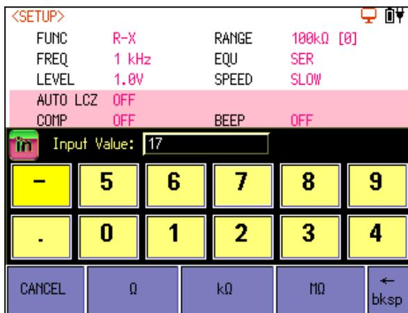
Note: If the touch screen is turned off in the system, when the input box is activated, the touch screen is automatically enabled for touch screen input.
