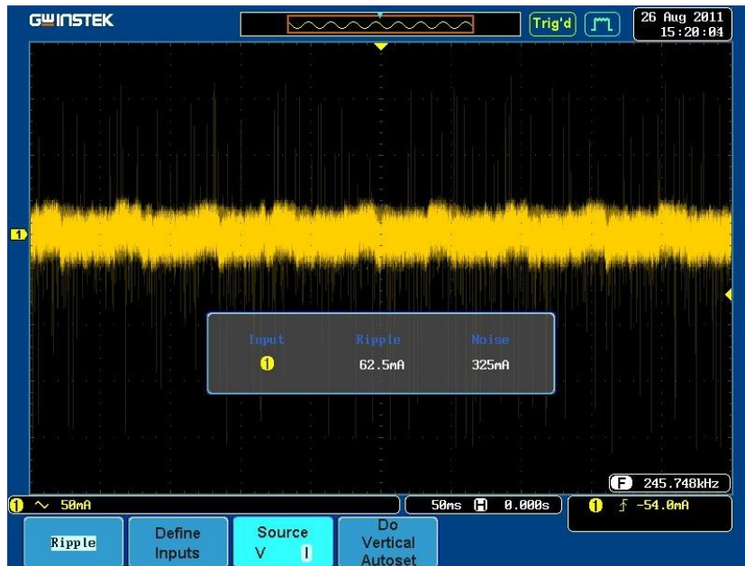
Figure 8: Ripple/Noise diagram of measurement results
