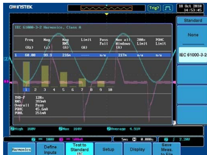
Figure 5: The GDS-3000 Harmonics function
