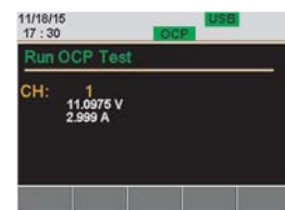
Result: Final DUT Output Status Before Entering OCP
