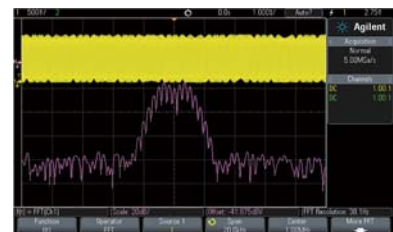
KEYSIGHT DSOX2000A - FFT Display
