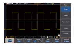
The GDS-1000B series oscilloscope is equipped with diversified trigger functions, including Edge Trigger, Delay Trigger, Pulse Width Trigger, and Video Trigger. Engineers, based upon different waveform measurements, can select different trigger functions to lock waveforms in order to identify the root cause of the complicated circuit designs to save development time and to accomplish tasks.
