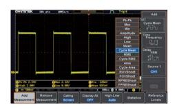
The GDS-1000B series oscilloscope is equipped with 36 different automatic measurement parameter functions. Users, after obtaining measured waveforms, can select different measurement parameters from Measure key according to different measurement requirements. The GDS-1000B Series shows simultaneously eight sets of different measurement parameters on the bottom of the
