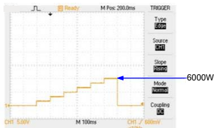
PEL-5006G-150-600 Turbo mode OFF OPP Pstep 50W, Pstep 6000.0W real test waveform
