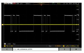
5. At this point, after the oscilloscope's Channel 1 probe contacts the test point, user will observe the waveform. If the yellow waveform does not match the reference waveform, it may indicate a potential issue or abnormality in the circuit.
