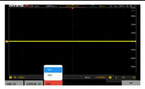
4. The current test item number and name will be displayed at the bottom of the screen. The gray waveform represents the stored reference test waveform.
