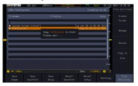
10. After completing the copy process, rotate the "VARIABLE" knob on the front panel and select the internal disk. Verify that the contents of the "TestExpress" directory have been successfully copied to the internal disk.
