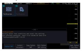
3. After launching the APP, users will enter the first-level menu. Press the "Start" button at the bottom left of the screen, and a list of "Test Object Models" will appear. In this example, sequentially select "MB\_01", "ERROR\_01", and "TP1". Press the "4" button at the bottom right finally to start the process and recall the settings and waveform stored in TP1.
