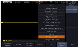
After the setting is completed, users can run the selected APP directly by pressing the "µPy/Exit" button on the panel.
