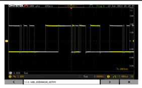
6. Press the ">" button to move to the next test item. If the test waveform matches the reference waveform, the user can proceed to the next test item.
