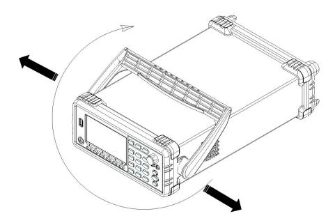
2. Further remove both the front and rear protective rubber casings away from unit as the figure below shown.
