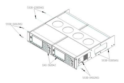
Hybrid unitsIn addition, 2 units of varied models can be assembled withapplicationthe rack mount together to form the hybrid application. Herewe take GDM-906X and DAQ-9600 for example as followswhere the front plate will be of no use and thus dismissed.
