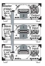
The PEL-2000A Series allows multiple mainframes to be linked together with standard MIL 20-pin connectors to provide higher power load capacity. A maximum of 5 mainframes, including one master and 4 slaves, can be chained together to give a 7kW load capacity for high current and high power applications
