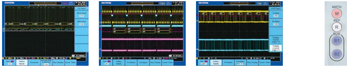
I 2 C Serial Bus Analysis Software SPI Serial Bus Analysis Software UART Serial Bus Analysis Software The GDS-3000 Series provides two dedicated keys in the front panel for two sets of setting recall
