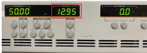
Figure 8.25 APS-300 voltage is bucked down to 13V
