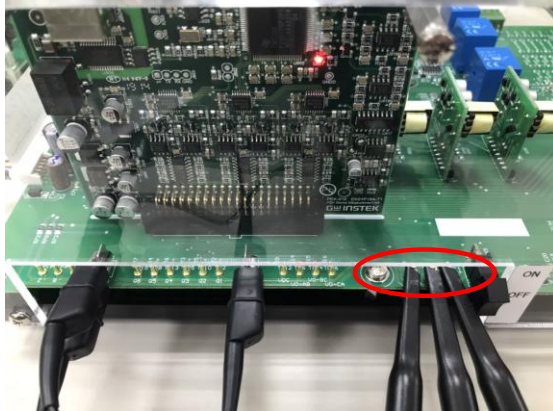
Figure 7.7 Oscilloscope test leads wiring
