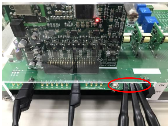
Figure 6.7 Oscilloscope test leads wiring
