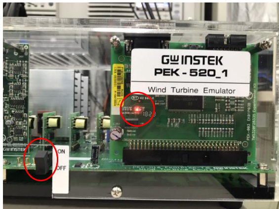
Figure 3.6 DSP normal status with light on
