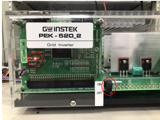
Figure 2.6 DSP normal status with light on
