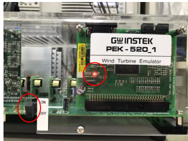
Figure 4.10 DSP normal status with light on
