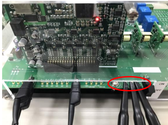
Figure 4.11 Oscilloscope test leads wiring
