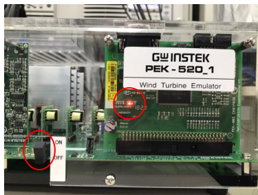
Figure 8.6 DSP normal status with light on
