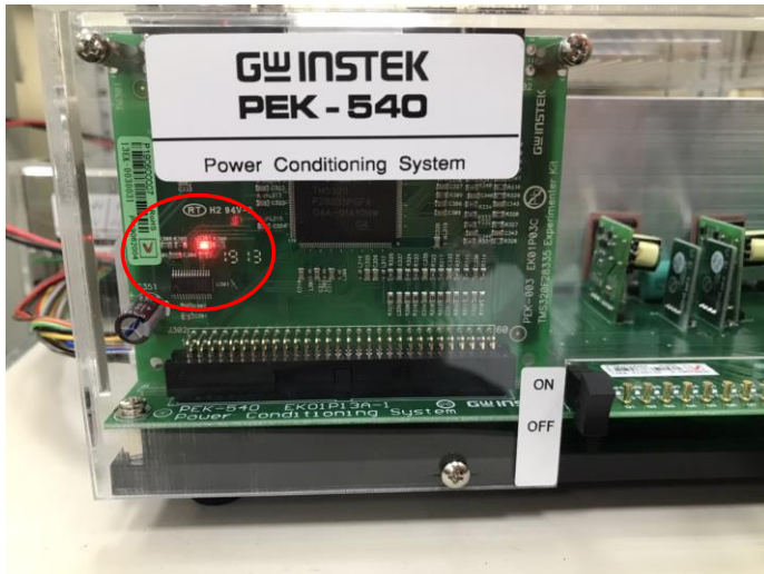
Figure 3.7 DSP normal status with light on
