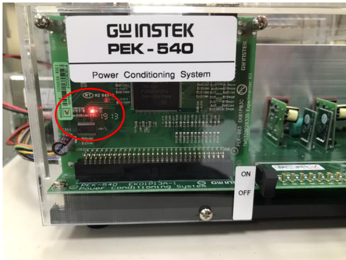
Figure 2.7 DSP normal status with light on
