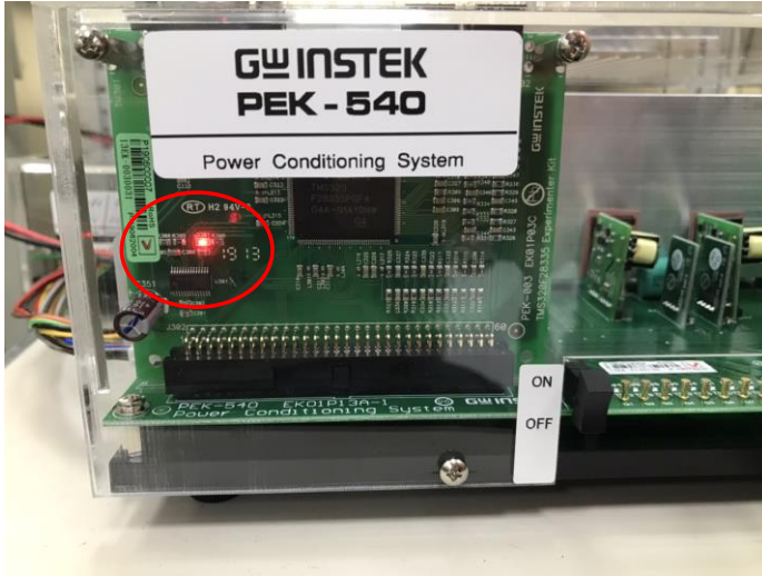
Figure 6.10 DSP normal status with light on
