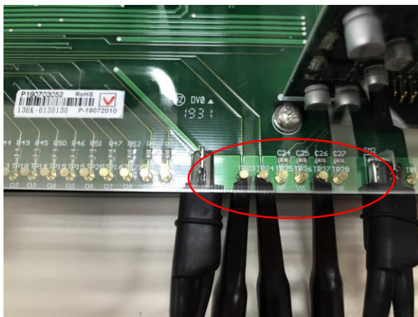
Figure 2.8 Oscilloscope test leads wiring
