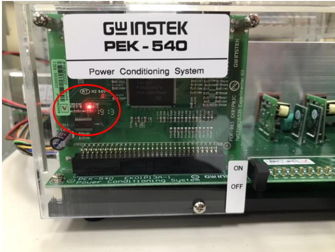
Figure 1.7 DSP normal status with light on
