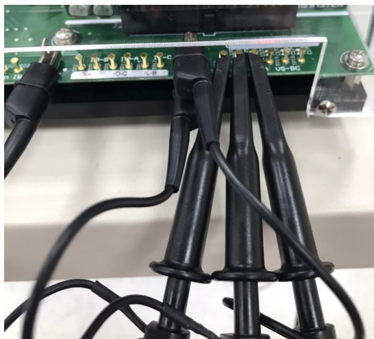
Figure 6.8 Oscilloscope test leads wiring
