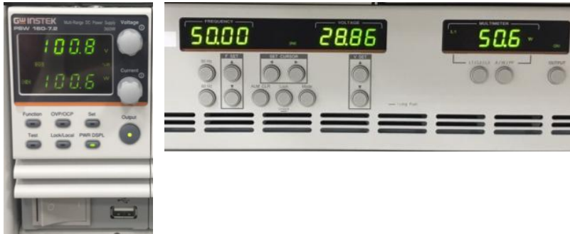
Figure 3.23 The power state of PSW and APS-300 when full load After the experiment, power off PEK-550 followed by turning off PSW, APS-300 and GPL-500.
