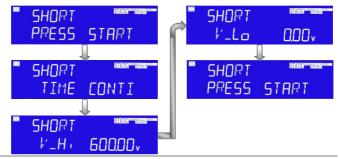
Set the short test time, the LCD display show "SHORT" on left 5 Digits LCD display, shows "TIME" on middle 5 digits LCD display, right 5 digit LCD
