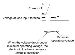
Waveform example: Generate unstable oscillation
