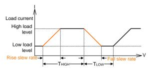
The dynamic waveform can also be set up via the optional computer interface. Dynamic waveform settings made from the front panel of the load module can also be saved in the memory of the PEL-5000C series Electronic Load. For the store/recall procedure and the computer command set please refer to the relevant operating manual for the PEL-5000C series Electronic Load.
