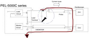
If the probes connection is reversed as shown above, a large current would flow through the probe and the internal circuitry of the oscilloscope is likely to be damaged.
