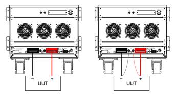
Typical connection of PEL-5000C series load module
