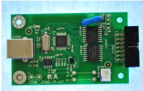
Figure 3.15 USB_JTAG burning circuit
