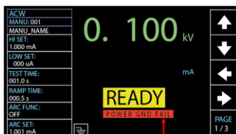
POWER GND FAIL Message
